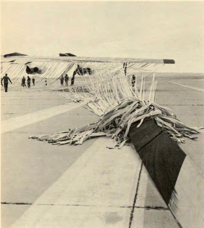
Upper Photo—Test aircraft has just entered the net. Note rubber supporting tubes draped over wings. Lower Photo shows enormous size of tape attached to nylon webbing—0.40 inch thick by 18 inches wide.
